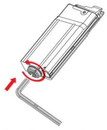
1.Use a 6mm hex wrench, small nose plier or a coin to unscrew the end cap at the magazine bottom in anti-clockwise direction.
