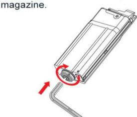
3. Place the end cap back and tighten it in clockwise direction. Turn the end cap quickly once hear the gas leaking sound until the sound stop.\*For safety reason, release all the pressure inside the magazine before storing.\*
