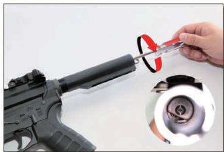
1. Remove the stock. Remove the screw with a Phillips head screwdriver in the stock tube.
