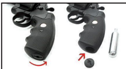
1. Grasp the grip tightly and use a HEX key or coins to unscrew the end cap anti-clockwise to open. Insert the CO2 cartridge, screw back tightly the end cap.
