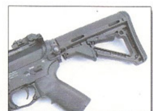
7. Install the stock back onto the pipe. Installation completed
