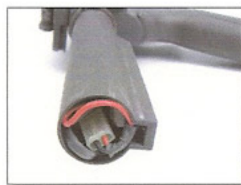
5. Place the plugs and wires back into the pipe
