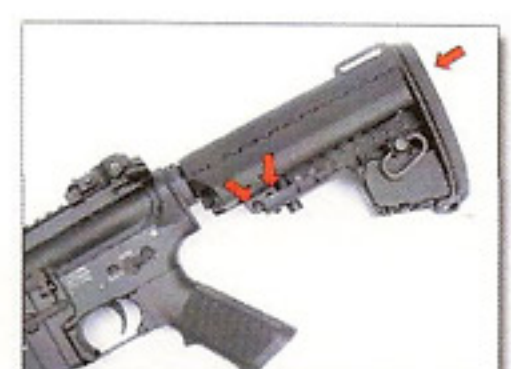
11. Fix the buttpad and three screws indicated to complete installation.
