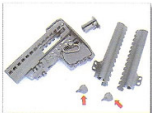
4. Remove the covers from the accessory compartments.
