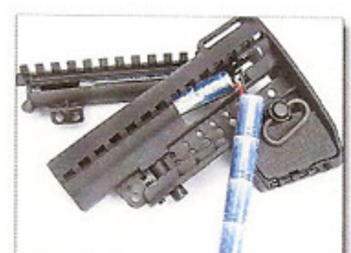
7. Put the other side of battery across the stock as shown.
