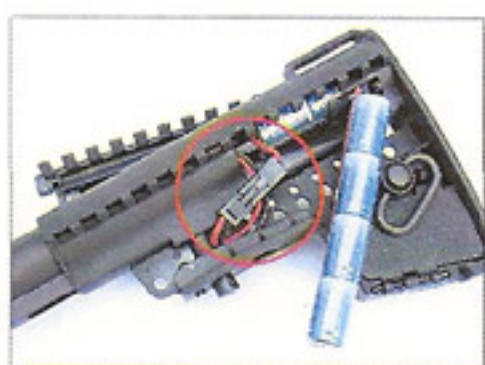
9. Connect the plug as shown. Place the wire and plug inside the stock pipe and make sure the stock can move smoothly.
