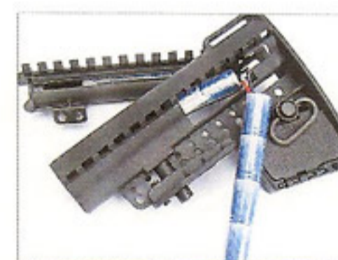
7. Put the other side of battery across the stock as shown.
