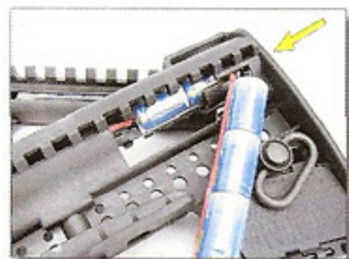
8. Place the single piece battery in the middle of the stock, and put back the stock cover (yellow arrow) to hold the battery on position.
