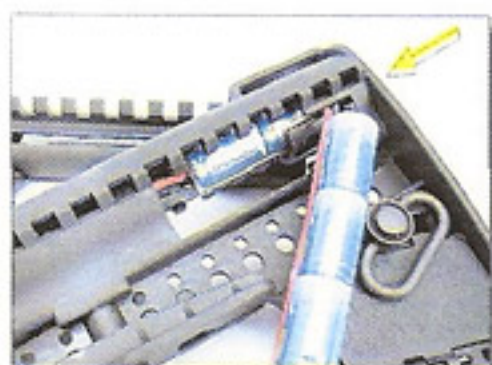
8. Place the single piece battery in the middle of the stock, and put back the stock cover (yellow arrow) to hold the battery in position.
