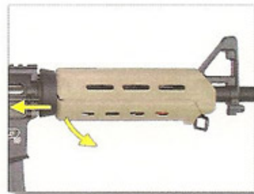
1. Pull delta ring backward and take the lower handguard off from AEG.
