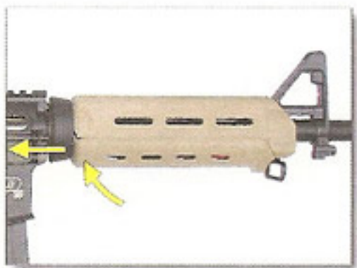
4. Install the lower handguard back on. Installation completed.
