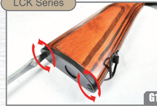
Remove screws & detach the Butt plate.
