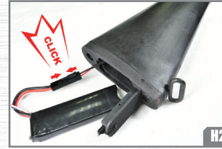
Connect and put a battery into the stock. Close the lid.
