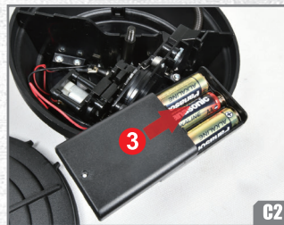
Install 3 AA alkaline batteries into the battery box. Turn the power switch ON. Put the butt plate back and fix the screw.
