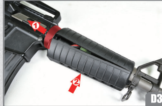
Connect a battery. Attach the handguard by steps.
