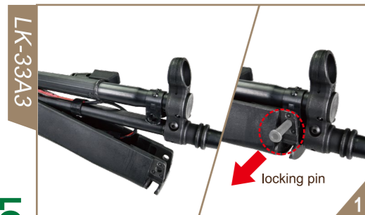
移除護木固定插銷 Remove the locking-pin in front of the handguard.
