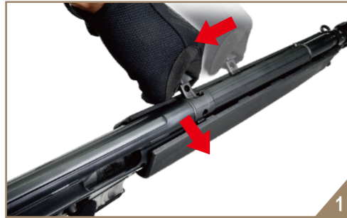
向後拉動槍機拉柄，固定於缺口中 Pull back the cocking lever and stabilize it at the notch.
