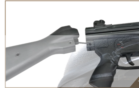
卸除後托插銷及槍托總成 Remove the locking pin and detach the stock assembly.
