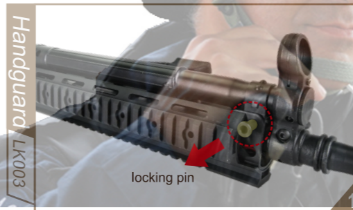
移除護木固定插銷 Remove the locking-pin in front of the handguard.
