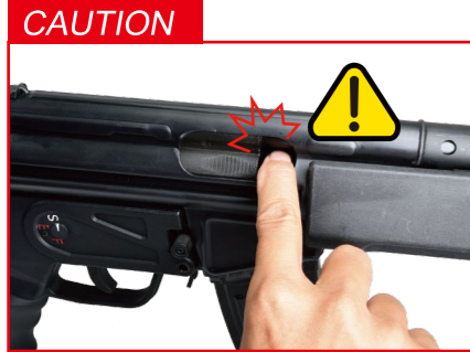
調整HOP UP時慎防夾傷手指 Be careful not to pinch your fingers while adjusting HOP UP.
