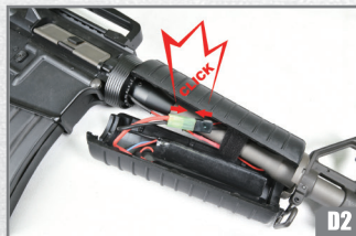
Push the handguard ring backward and remove lower handguard.
