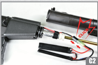
Press the button(1) & Rotate the Handguard (2) then forward remove it.
