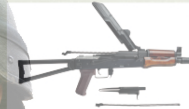
10. 再依序組裝槍機組、上蓋即組裝完成。 Assemble Bolt Carrier Set, Top Cover in order and completed.
