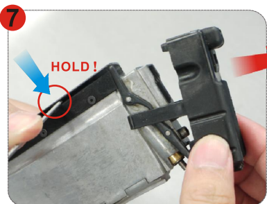
7 將舊款上蓋與彈匣分離 Release the old cover.
