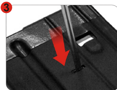
3 壓下上蓋卡榫(兩側) Press the catch (both side)
