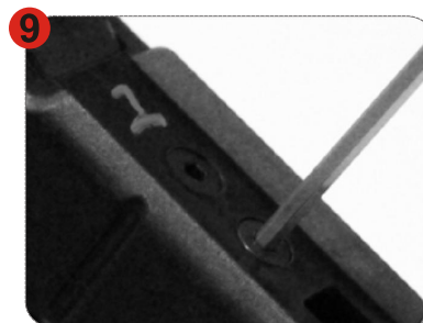
9 將上蓋與彈匣結合，並鎖上螺絲 Put the new cover on and fasten the screws.
