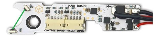
Sector gear phototransistor (sensor) and IR LED diode work in pair as a barrier switch. When sensor and diode cannot "see" each other, it means that the sector gear cut-off cam is between them. Perun AUG is using information whether the cam can be seen or not, to determine which gearbox cycle phase is currently taking place. Photo below shows the line between the sensor and the diode.
