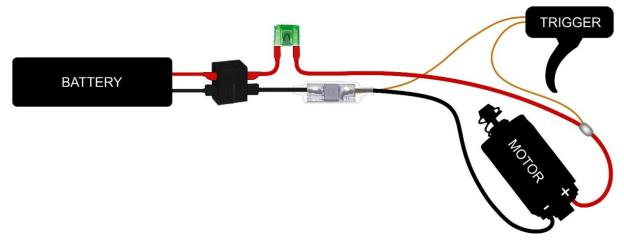
This is the standard installation scheme. If you are using a version 2 gearbox and would like to make it easier, please have a look at the "One signal wire" scheme. Before cutting the wires, make sure you got the lengths right!
