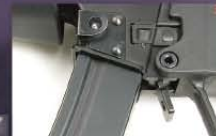
4 Set the magazine upward. Connect firmly till a click sound is heard.
