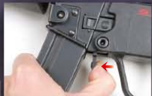
1 Pull the lever forward to release the magazine.
