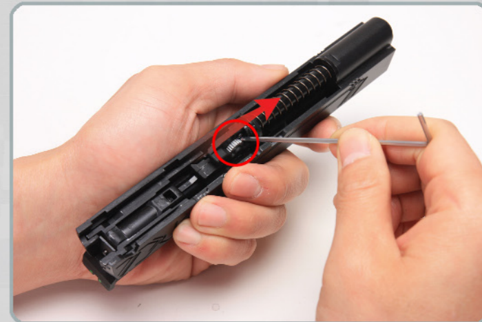
No Enough Hop-up To increase the Hop-UP setting , rotate the Hop-Up dial towards Hop.
