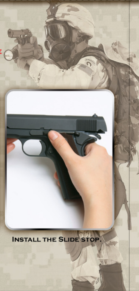
PULL BACK ON THE UPPER SLIDE AND HOLD IT IN PLACE AS SHOWN ABOVE
