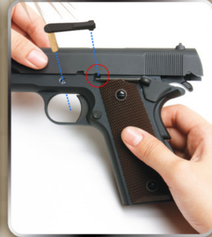
PULL BACK ON THE UPPER SLIDE AND HOLD IT IN PLACE AS SHOWN ABOVE
