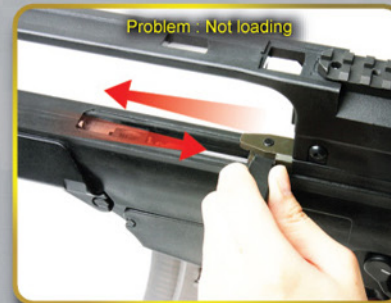
Pull the Charging Handle to rear and release it.
