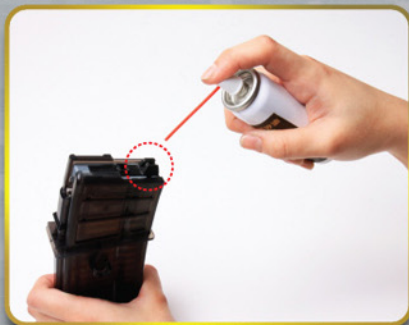
Use Airsoft Safe Silicon to lubricate the hop up chamber and Magazine lip. Use silicon lubricant sparingly..
