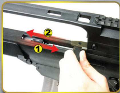
Pull the Cocking lever to rear and release, then will ready to fire.
