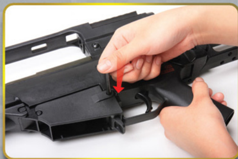
Insert the locking pin in front of lower receiver.
