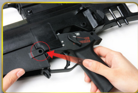
First, locking the front of lower receiver.
