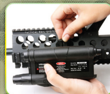
Reinstall the external battery case.
