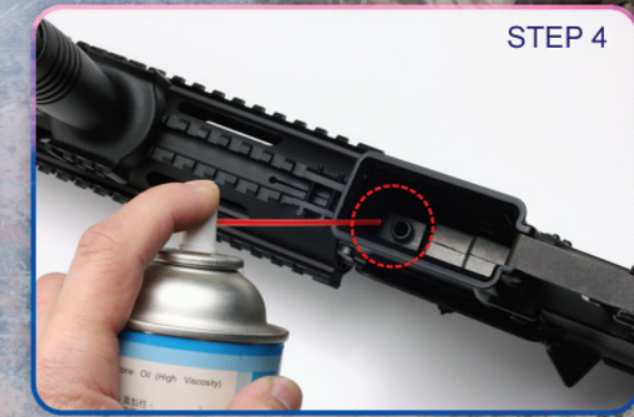
Use Airsoft Safe Silicone to lubricate the hop up chamber. Use silicone lubricant sparingly..
