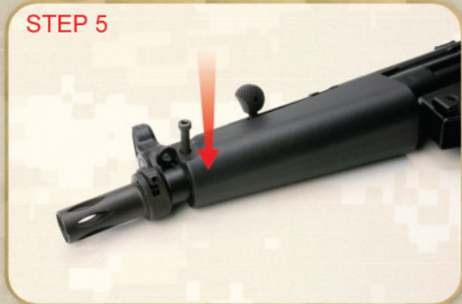
Insert the locking pin.
