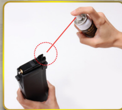
Use Airsoft Safe Silicone to lubricate the hop up chamber and Magazine lip. Use silicone lubricant sparingly..
