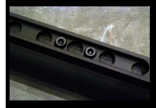
However, in the event that the screws are over tightened, the Recoil Pulley Gear Stand may warp its shape. The goal is to aim for around the 9 O'clock position.
