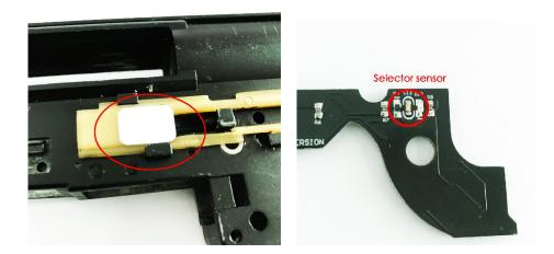
具体贴纸位置以实际情况为主,需要反复调整,确保单连发 位置准确 The specific position of the sticker is mainly based on the actual situation, which needs to be adjusted repeatedly to ensure the accurate position of full-auto and semi-auto.
