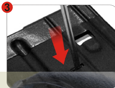
3 壓上上蓋卡榫(兩側) Press the catch (both side)
