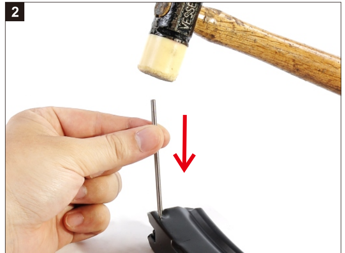
2 將彈匣固定梢敲出。 Remove the pin by tapping it out.
