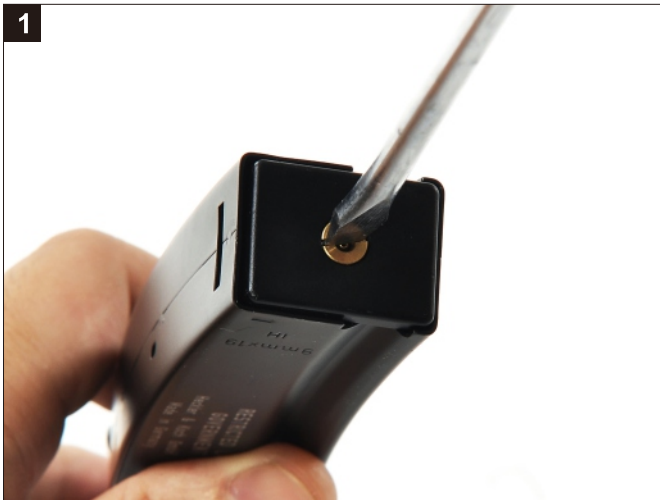
1 將彈匣內氣體釋出，並以工具卸下灌氣嘴。 Make sure the magazine is empty without gas before remove the Injection Valve.
