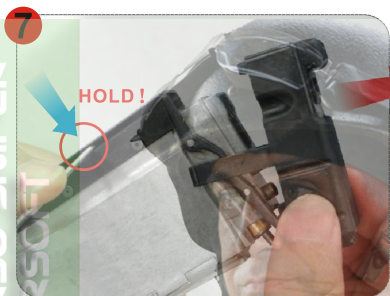
7 將舊款上蓋與彈匣分離 Release the old cover.
