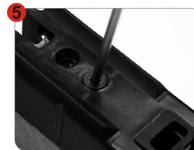
5 卸下螺絲 Release the screws.
