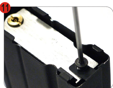
11 鎖上螺絲 Fasten the screw.
