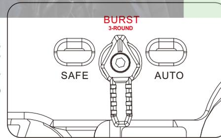
Set selection lever in SEMI mode, pull and HOLD the trigger for few seconds, the TRIPLE "BEEP" sound will be heard, Now in 3rd firing mode. If you repeat the operation again, system return to default start mode.
