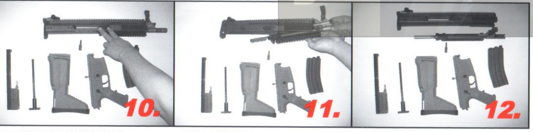
使用梅花扳手轉開左右側槍管結合螺絲 Remove the two barrel fixed (star) screw on both side middle of upper receiver. 向前向上分離槍管總成 Push forward the barrel sets forward 4.5 cm and pull up to take out the barrel sets. 大部分分解完成(反向即可組裝恢復) Complete.(Please reverse step to complete installation)
