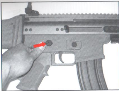
左側位置 The selector button on left side for left hand shooter.
