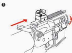
After adjustment, pull back the charging handle & close the ejection port cover
