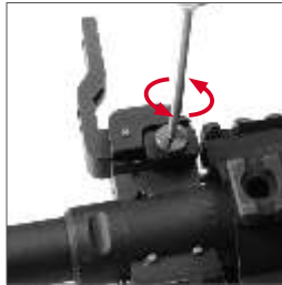
To release the front sight: Unscrew and take the fixing screw off and remove.
