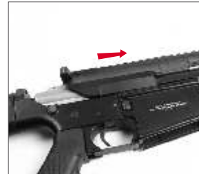
Move the upper receiver forward till separate with lower receiver.
