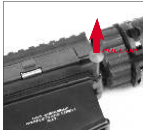
Pull the receiver pivot pin out.
