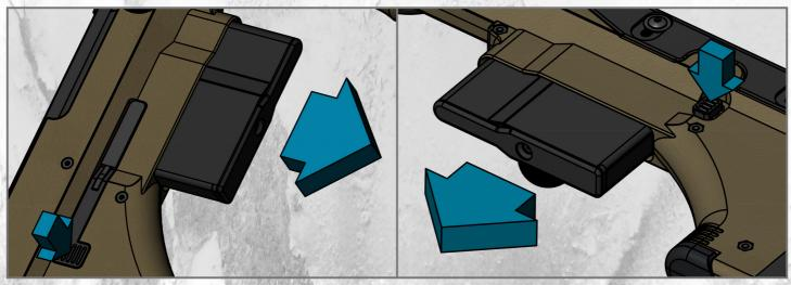
To remove the magazine, press the magcatch button and pull down the magazine.
