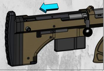
Insert the dust cover into the ejection window, then slide it backward. Use the bolt handle to ease the installation.
