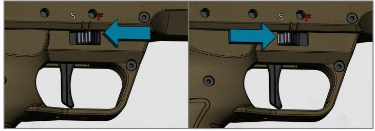
Slide the safety button (left or right) to «S» position to engage the safety.
