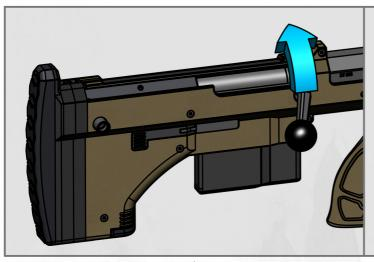
Lift up the bolt handle (make sure the bolt is not already armed to avoid double feeding).
