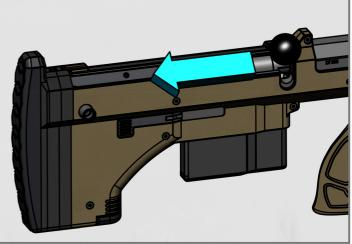
Move the bolt backward to compress the spring and lock the piston sear (until it clicks).
