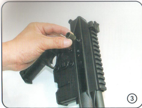
取出拉柄，槍機即可取出 Remove the Charging Handle and the Bolt Carrier Group.
