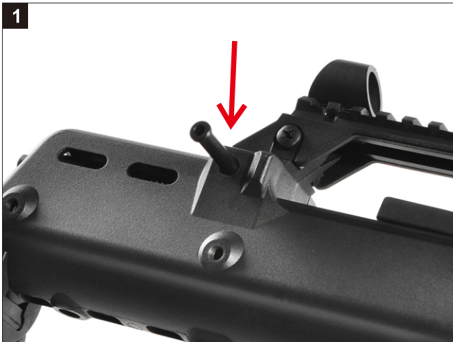
1 移除護木固定梢。 Remove the Locking Pin from the Handguard.
