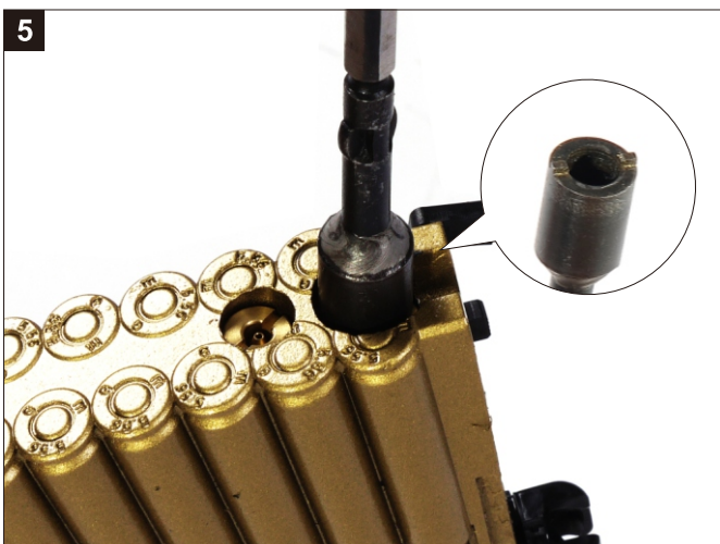
以專用工具將彈匣氣閥卸下。 Remove the Valve by using a specific tool.
