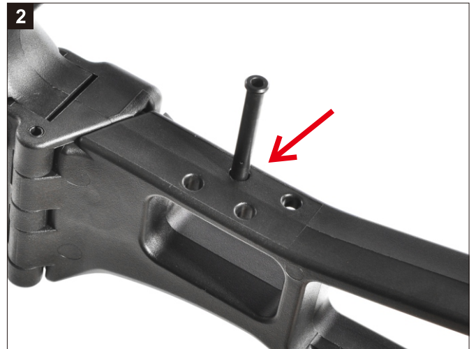
2 插梢可置放於槍托之容納槽。 The Locking Pins can be stored in the hole in the Buttstock.
