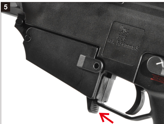
5 按壓彈匣釋放鈕，並將彈匣井向下取出。 Push the magazine catch, swivel the Magwell downward and detach.
