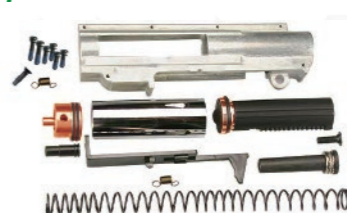
Upgrade Upper Gearbox D (M120 Spring, Aluminum Cylinder & Oversized Piston Head, 4 Opening Oversized Cylinder) 升級上齒輪箱組 -D (M120 彈簧; 加大鋁活塞頭組; 開 4 孔加大氣缸) MA-54
