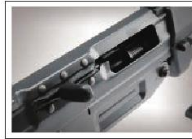
Pull charging handle to the end and fix it
