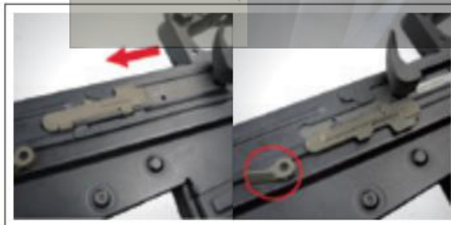
The charging handle can be fixed at the rear by pulling it back and raising the charging handle catch
